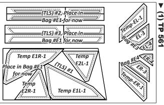
**NOTE - Reusing Templates:** Templates and (TLS) are repositioned on the cut strips to achieve the number of cuts required in the cutting Instructions. Please read carefully to ensure the correct # of pieces are stacked beneath each Template before cutting.
