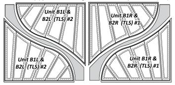
**NOTE** - You will need to reposition the (TLS) with each cut. Only (1) (TLS) is provided with each booklet. Repositionable Glue applied to the backside of the paper template holds the paper in position during the cutting process.
